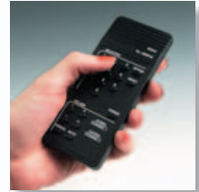
Infrared remote control with selection buttons
