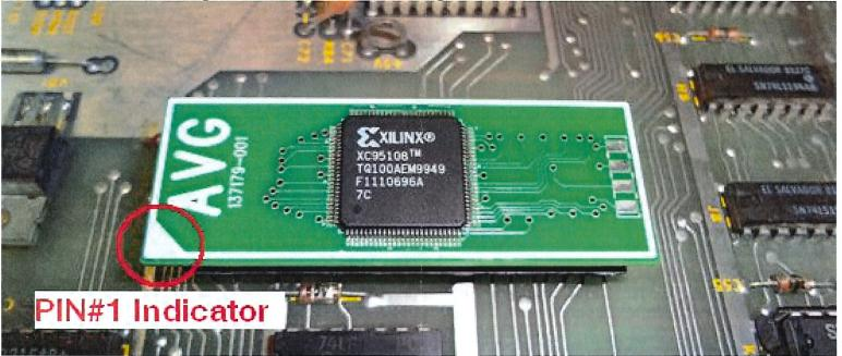
Note: The Xilinx chip on the board can be easily damaged if the game board is stacked with other game boards. The chip has fine legs that can be easily bent if brushed against. To further protect the new chip hot glue or two part epoxy can be applied to the legs around the Xilinx chip. This will have no effect on the operation of the chip but will help protect the chip from outside handling/stacking of boards.
