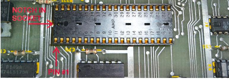
2) Install the new chip as shown with pin #1 matching pin #1 on socket. Verify all pins are aligned in the contact areas and press firmly down on the chip.
