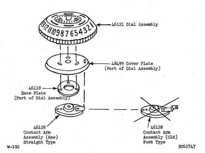
After installing the new contact arm assembly, assemble the contact cover so that the slot centers with #1 on the dial, and tighten the screw opposite #19 on the dial. The other two screws should be in position but remain loose until properly positioned. (See sketch below.)
