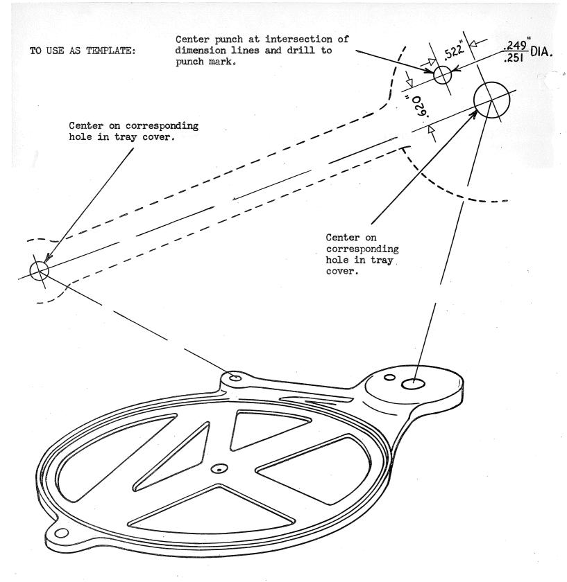
NOTE: Record Tray Cover, Part No. 27245, as installed on Models 1017-A, 1080-A and 1100 Phonographs, has a hole to accommodate the locating stud on the stabilizer arm. A few Model 1015, 1017 and 1080 Phonographs will be encountered on which this tray cover, with the hole already drilled, has been used. In such cases, drilling of the cover will not be required.
