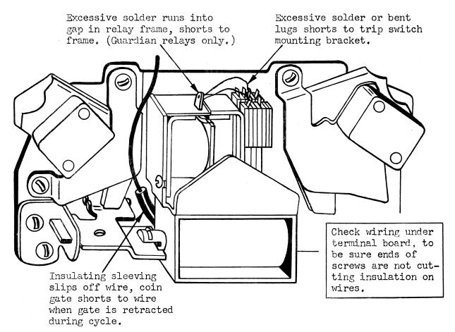
After clearing, all relay contacts in Bar Boxes and Master Unit should be cleaned to compensate for excessive arcing due to above conditions. These items are being carefully checked in all present and future production.
