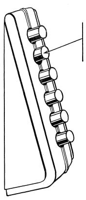
Binding may occur at opening in selector switch casting due to selector buttons rubbing on casting.
