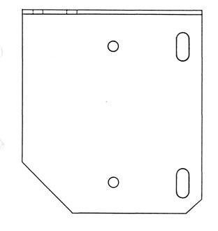
A Mounting Bracket is available for purpose of installing two Micro Switches in the Model 1250 tone arms circuit. This may be ordered as Part No. 54932.
